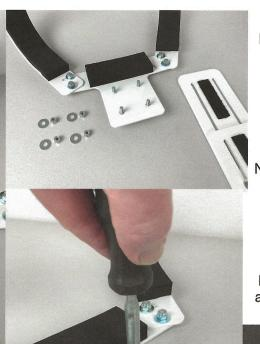
Now let's attach the vertical brackets to the Yoke with the washers and lock nuts.
