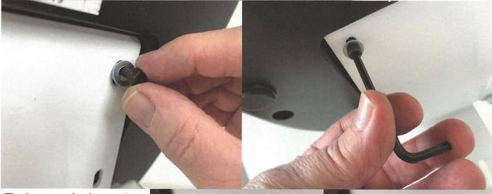
The longer pair of mounting bolts are provided as an option. You may or may not need to use them but they're there in case you'd like an added layer of 'security' in attaching your controller to the Walkabout carrier.
