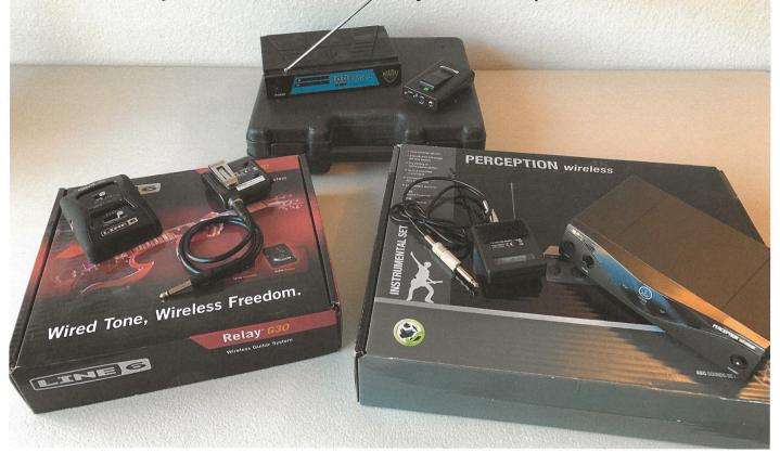
Most guitar style wireless transmitter systems have two main components. The transmitter is often a small 'body pack' that guitarists will attach to their belt or the guitar strap. The 1/4" male plug is connected to the (mono) audio output of your controller, unless you're bold enough to operate two simultaneous wireless systems for a full stereo effect - again totally up to you.
