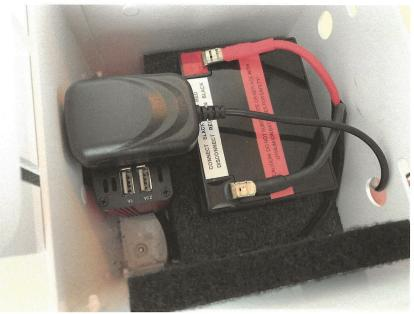
Now you can connect the ac adapter plug to the power outlet of the inverter.
