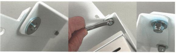
Now secure the top bracket to the side bracket with washers and lock nuts as shown to the left. No need to over tighten the lock nuts. The nylon sleeve keeps things locked in place.
